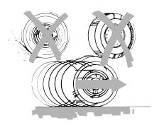
The front wheels have to be turning in order to steer the vehicle. Rapid pumping of the brake pedal will help you slow the vehicle and still maintain steering control.
